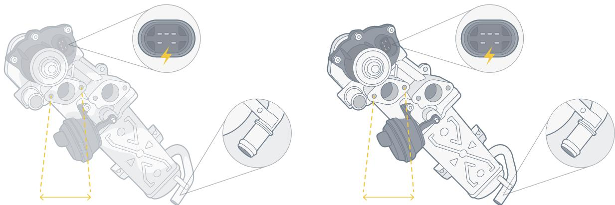
Make sure, that you have received the correct valve by comparing measures on connecting flanges, pipes and plugs.
