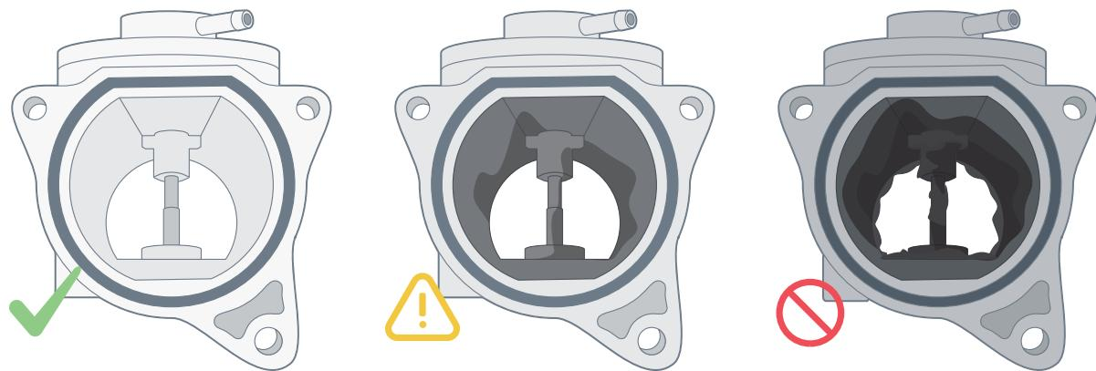
Soot may have built up excessively in manifold, connecting pipes, cooler, by-pass valve and on throttle body. Based on old EGR valve condition (contamination level), please determine if cleaning EGR circuit is necessary.
