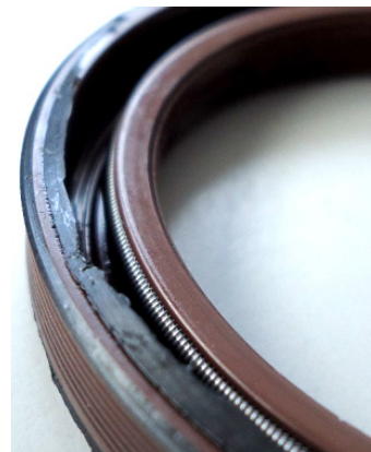
Sealant remains in the external diameter of the seal
