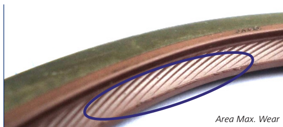
Seal perpendicular to the axis
