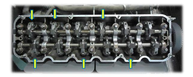
5. After adjusting all valves, proceed to the assembly of the rocker cover installing a new gasket (11031000) and perform the specified torque.
