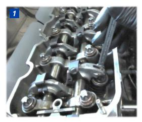
3. Tighten the nut for fixing the eccentric washer in the correct position while the gauge is introduced between the rocker and the valve head.
