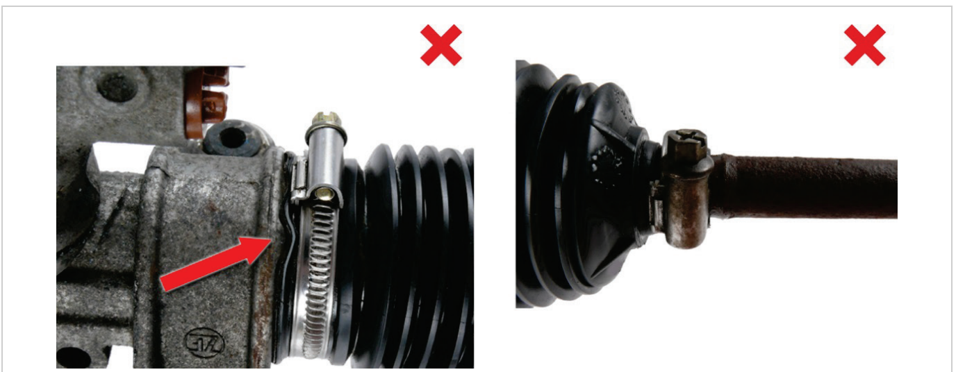
Fig. 7: Bypass: faulty sealing with hose clamps
