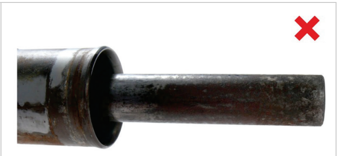
Fig. 4: Rack with corrosion
