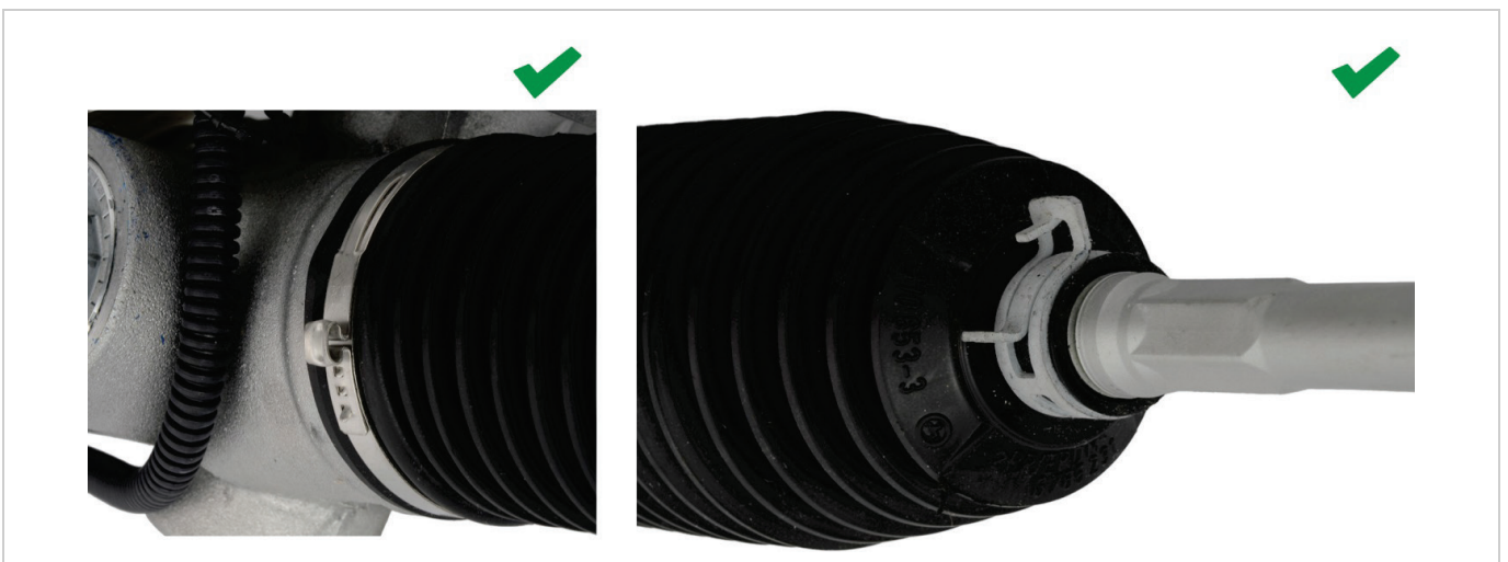
Fig. 6: No bypass: correct sealing with metal clamps
