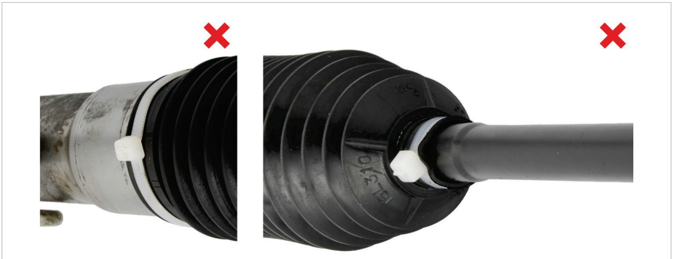
Fig. 8: Bypass: faulty sealing with cable ties
