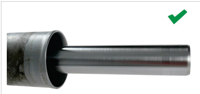
Fig. 3: Rack without corrosion
