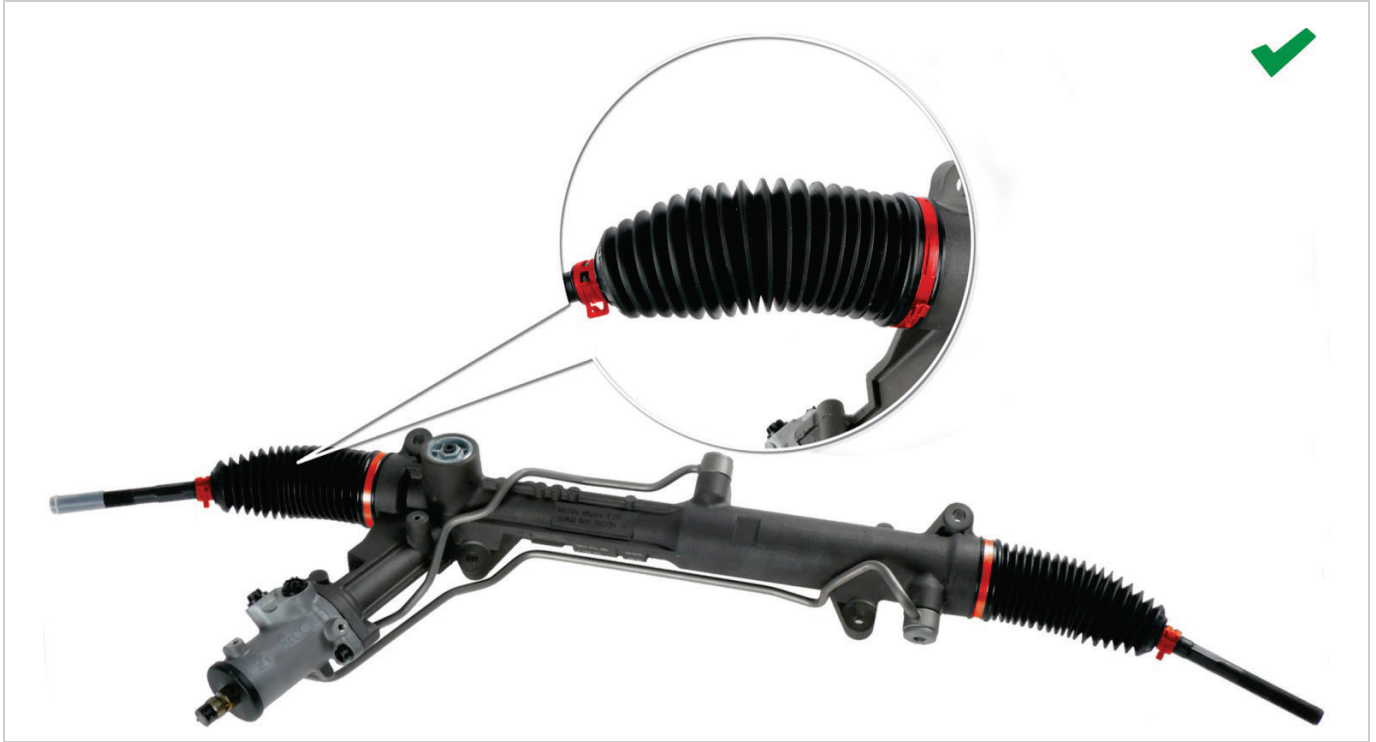
Fig. 2: Steering gear with hydraulic steering assistance: correctly fitted steering sleeves
