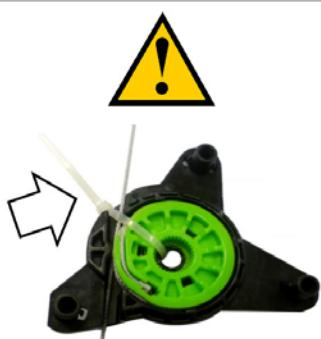
It is recommended not to remove the PVC gear clamp until mating with the engine in order to avoid possible unroll of the cable during assembly.
