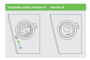
Fit both tensioner pulleys as specified in ESI[tronic]-M. When installing the new tensioner pulley (3), make absolutely sure to fully tighten the screw to the engine housing in order to release the load from the ground plate of the tensioner pulley. In version A, the ground-plate lug is to be well-locked at the notch (8) whereas version B comes without any lug to be locked at the ground plate.
