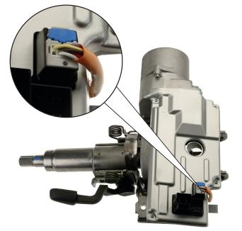
Steering column with external sensor connection
