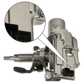
Steering column without external sensor connection
