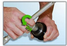
*Image 6:* You will notice an increasing spring force when the tool is moved in an anti-clockwise direction.
