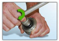
Image 5: The tool can be continuously turned in a clockwise direction with slight resistance.
