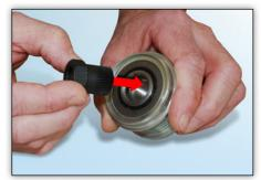
Image 3: The corresponding adapter is inserted into the overrunning pulley.
