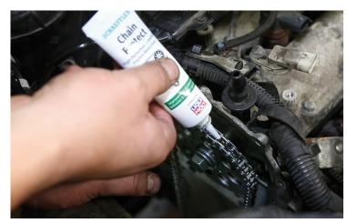
Photo 2: Schaeffler Chain Protect is applied to all timing chain system components during chain installation.
