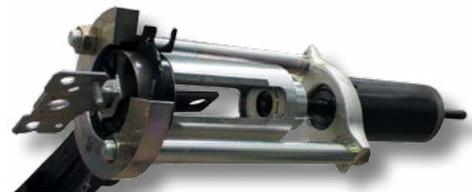
Of course, febi bilstein also offers the rear trailing arm bush kit as a ProKit (febi 43403) containing all the necessary screws for a professional replacement
