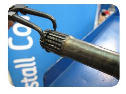
6. Expand and remove the circlip with circlip removal pliers.
