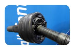
3. Press the new CV-Joint onto the shaft. Tap with a rubber hammer until the circlip locks into its groove in the inner race of the CV-Joint.
