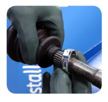
1. Put the short boot clamp on the shaft. Slide the boot on the shaft.
