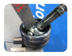
4. Cut the tracks of the inner race, in 2 o 3 positions by using a suitable cutting tool.
