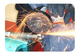
4. Cut the tracks of the inner race, in 2 or 3 positions by using a suitable cutting tool.
