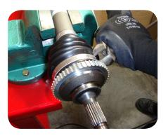
2. Place the driveshaft in a vice (with aluminum or protective jaws). Remove both the inner and the outer clips.
