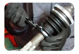
5. Fit the short and long clamp onto the CV-boot and tighten it with a suitable tool.
