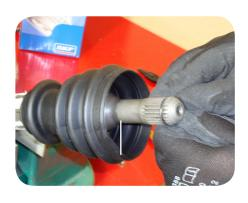
3. Press the new CV-joint onto the shaft. Tap with a rubber hammer until the circlip locks into its groove in the inner race of the CV-joint. Remove the hose clip.
