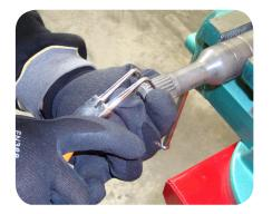
6. Expand and remove the circlip with circlip removal pliers.
