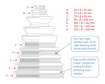
When fitting the universal boot onto the CV-joint, it is recommended to cut the boot to size after having tightened the clamp.
