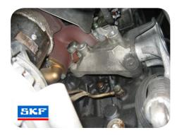
3. Remove the alternator bracket with the VKM 34032 tensioner attached to it.
