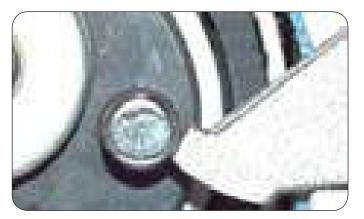
• Turn tensioner clockwise using an Allen key and slightly compress piston, remove the piston retaining pin and allow the piston to fully extend. Adjust the tensioner using a Dynometric (Torque) wrench.
