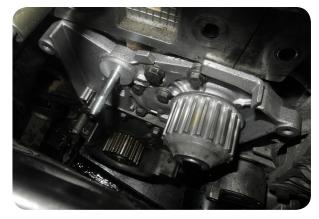
Water pump mounted with stud tightening
