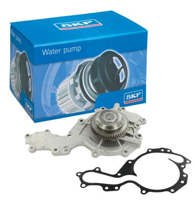
To facilitate easier mounting of the waterpump on this V6 engine, the current paper graphite gasket sold with the SKF pump for many years is replaced with a rigid stamped metal version.
