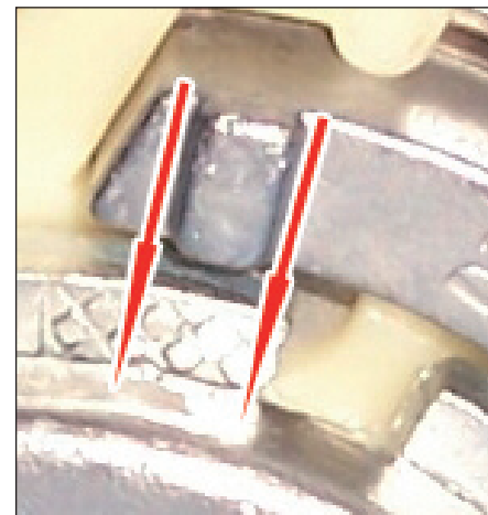
Fig. 5: Both notches are outside the cut-out (arrows) This setting must be corrected!
