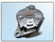
**Image 3:** Example of a broken 533 0017 10 tensioning arm
