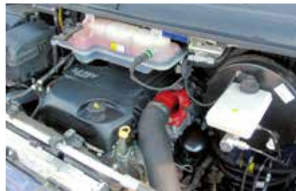
Regulating throttle (highlighted in red) in the engine compartment of an Iveco Daily 3.0 l
