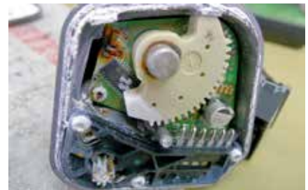
View of the interior of a damaged regulating throttle
