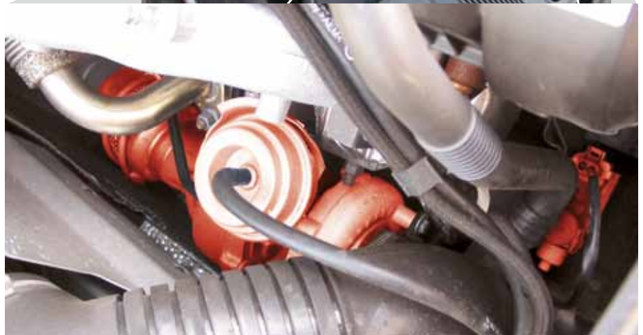
EPW and VTG charger (highlighted in red) in the Audi A4 TDI
