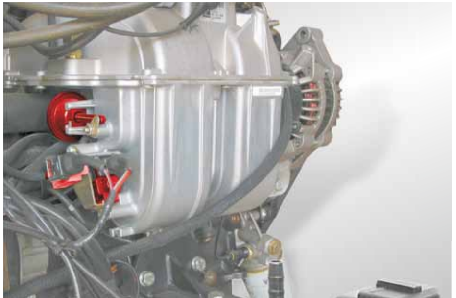
At the controlled intake manifold in the Opel Astra already two EUVs have been fitted (highlighted in red). One controls through the actuator above it (highlighted in red) the intake manifold throttles; the other switches the secondary air shut-off valve (not shown)
