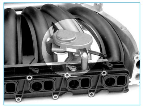
Intake pipe with EDM-i (highlighted)
