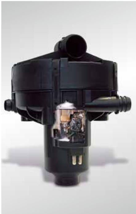
View into the secondary air pump (cut) with melting traces
