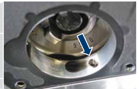
Example: On the Opel Vectra the lubricating oil feed is via holes in the flange
