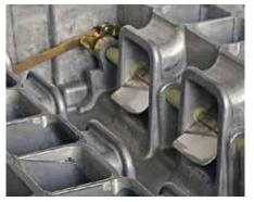
A view into the interior of a variable intake manifold
