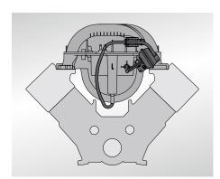
Variable intake manifold on a V engine
