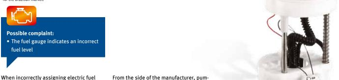
when incorrectly assigning electric fuel pump 7.00468.86.0 and vehicle, it is possible that the fuel level is indicated in the "opposite" way.
