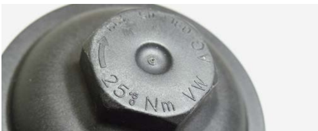
Figure 2: Torque specification on the housing cover
