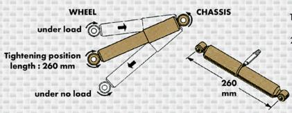
To facilitate installation, mark a reference guide on the new shock absorber, when the correct length of 260mm is achieved, the reference line should be used as a guide during the installation process. Ensure the reference line, lines up whith the dust shield before tightening the mounting bolts
